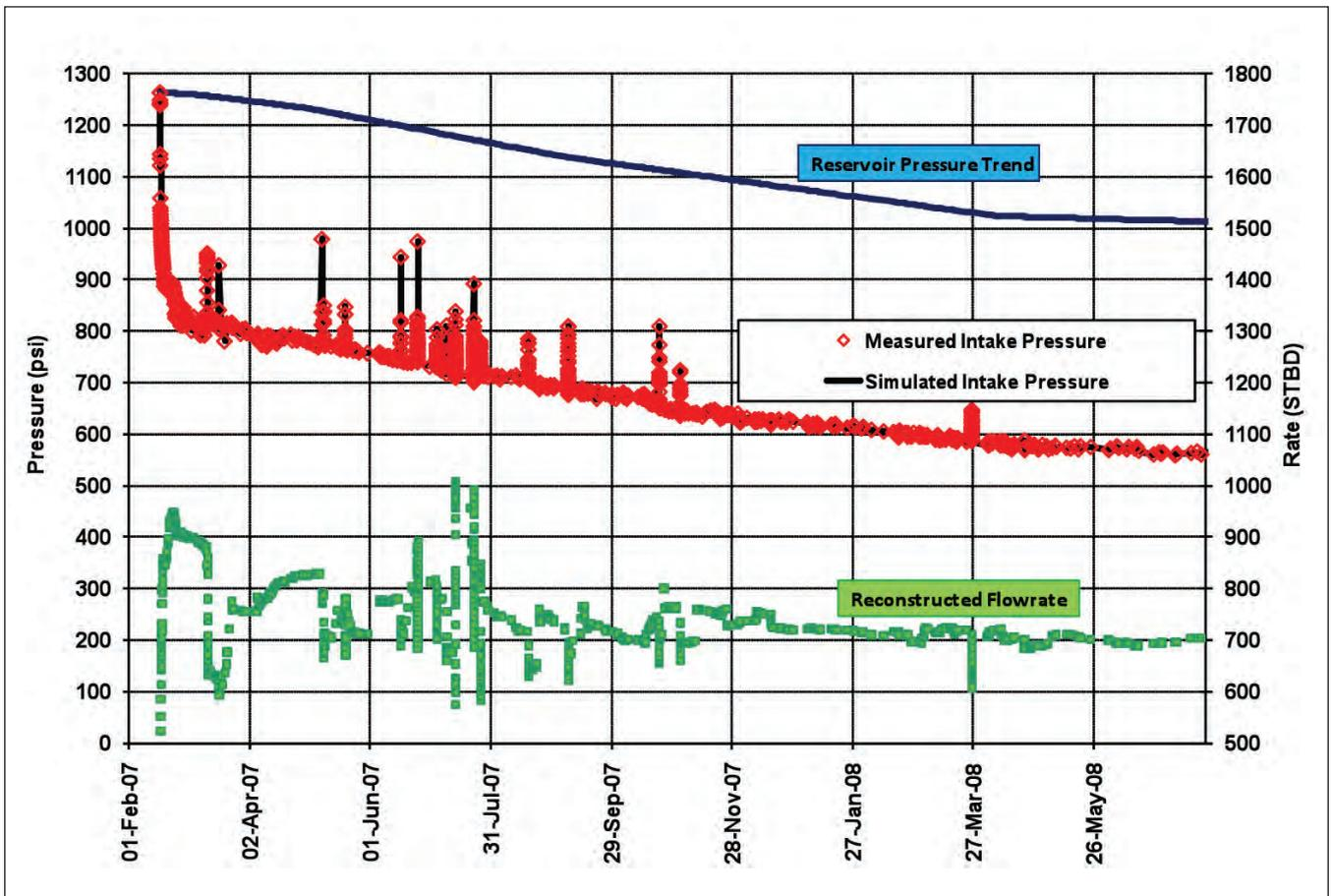
Reservoir pressure simulation using the superposition model shows the pressure decline in the drainage area. There is a match between the simulated and measured flowing pressure due to calculated flow-rate history that captures flow-rate transients.
