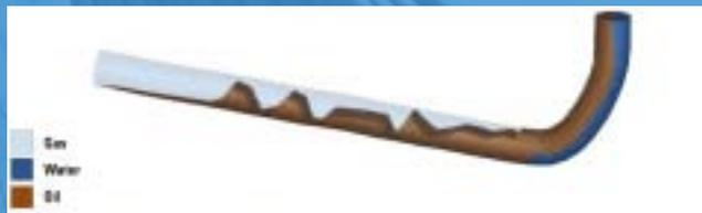
**FREEZE FRAME:** Instantaneous frame taken from a transient multiphase flow simulation done using OLGA.
