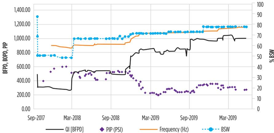
**Fig. 3.** Production profile of Well C, showing production variation in response to waterflooding.
