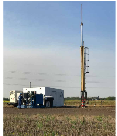
The CAMLift unit jack is installed directly on the wellhead, reducing preparation, installation, and servicing requirements.
