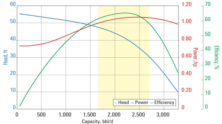
GN2100 pump curve for 60 Hz with  $sg = 1$ .
