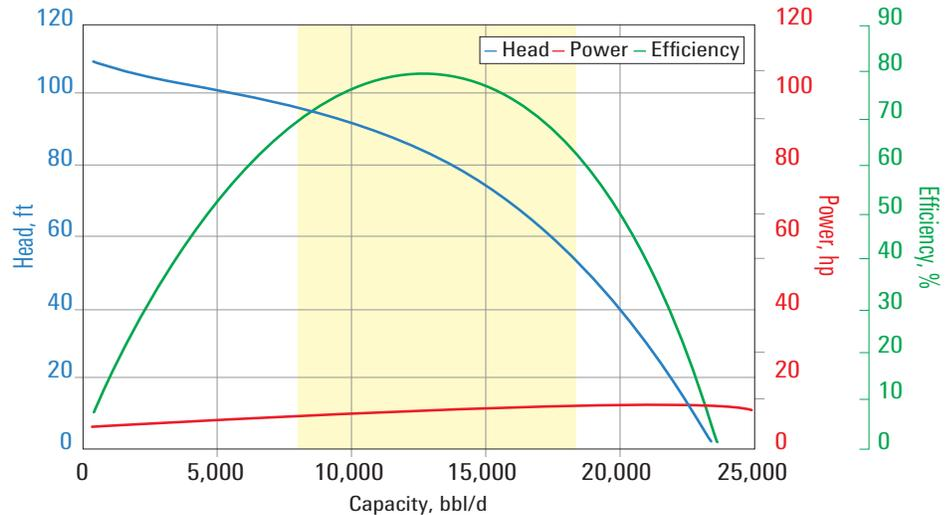
J12000N pump curve for 60 Hz with  $sg = 1$ .
