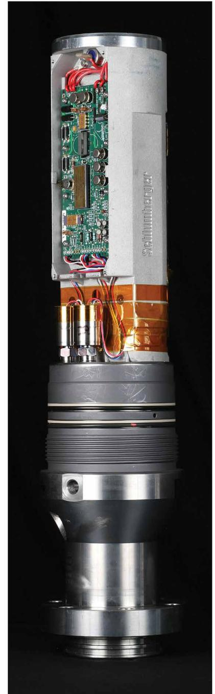
*Phoenix xt150 high-temperature ESP monitoring system.*
