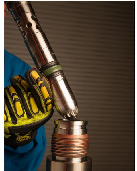
*Retrievable gas lift valves can be easily replaced using slickline to accommodate changing conditions or strategy.*
