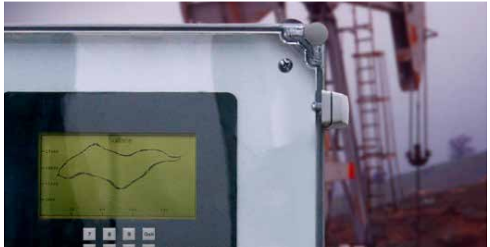
The RPC provides real-time surface and downhole dynamometer plots.
