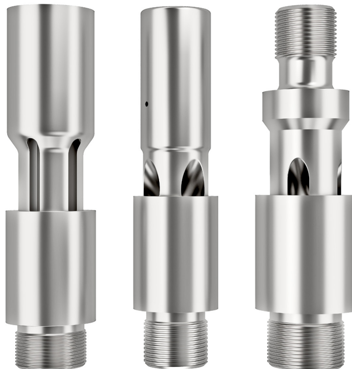
Sand diverters can be run with any hollow valve rod pump, insert pump, or tubing pump. Models designed to be compatible with each of those pump types are shown above, from left to right.
