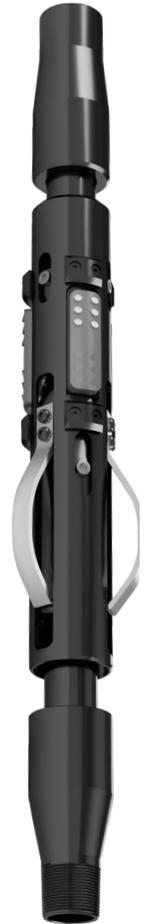
The slimhole tubing anchor has a smaller OD than the standard anchor, with large slips and slip protectors. Beveled couplings prevent sand from getting inside the tool.
