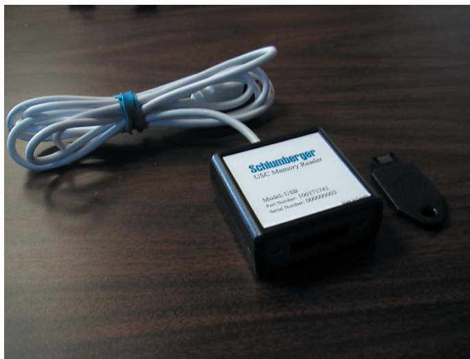
UniConn memory module and reader connected to a PC through USB port.
