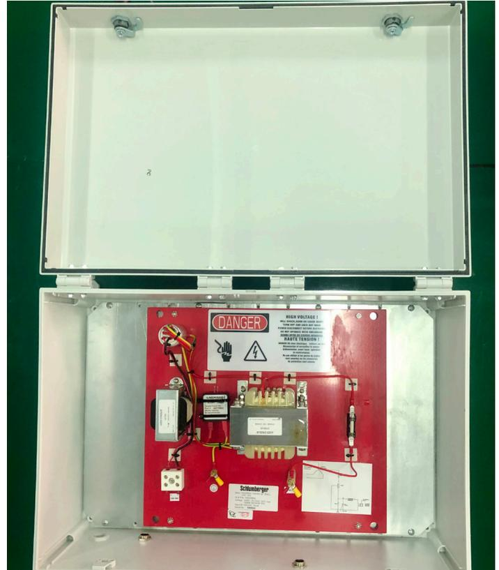
*Single-phase and three-phase surface choke panels prevent high-voltage alternating current from reaching the ESP surface controller while allowing data signals to pass, enabling ESP monitoring and control applications.*
