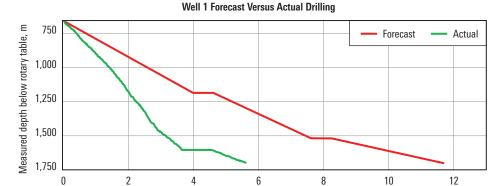
The EnduroBlade 360 bit and EnduroBlade 360 bit fitted with strategically placed Stinger elements delivered the 81/2-in section in half the forecasted time for Well 1, saving 6 drilling days.
