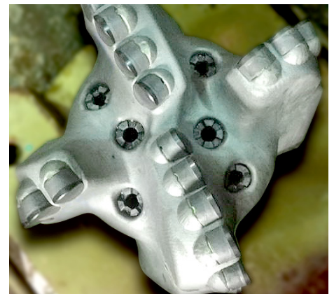
The HyperBlade bit maintained steerability and drilled faster than the high-ROP benchmark bit.
