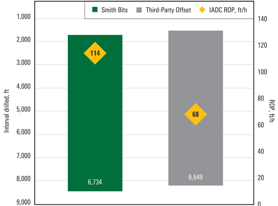
Synapse service designed a fit-for-basin bit that drilled 69% faster compared with the closest offset, drilling 6,734 ft at 114 ft/h vs. 6,649 ft at 68 ft/h.
