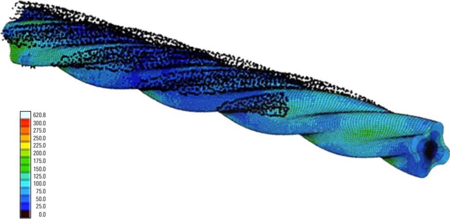
The i-Power service enables better elastomer and power section selection by incorporating data from the entire BHA including the bit and cutting elements, along with formation data.
