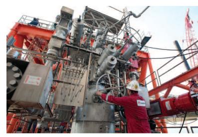
For the 25,000-psi production tree, the valve and choke, both critical components, and the tooling required for installation did not exist. (Source: Cameron)
