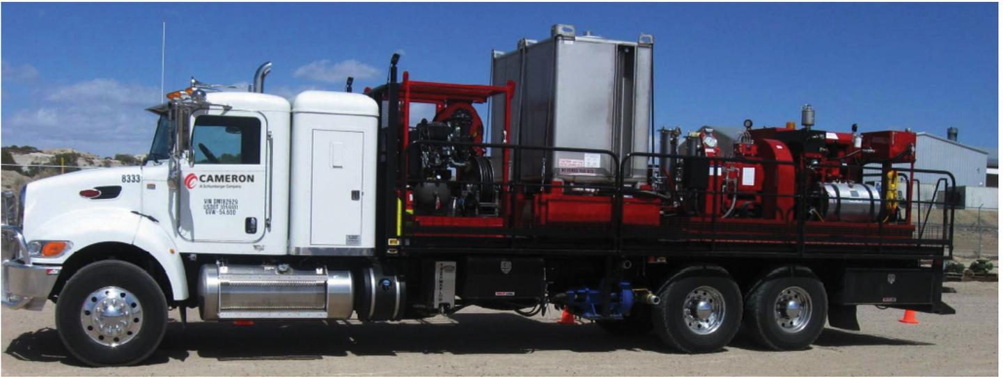
*Trailers are fitted to perform integrated field testing, power torque, and high-pressure greasing from a single platform.*
