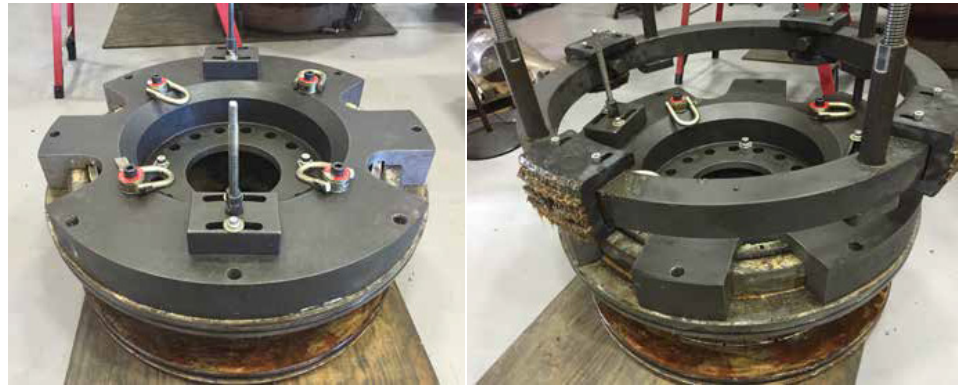
Assembly and disassembly tool for 18 3 / 4 DL annular BOP.
