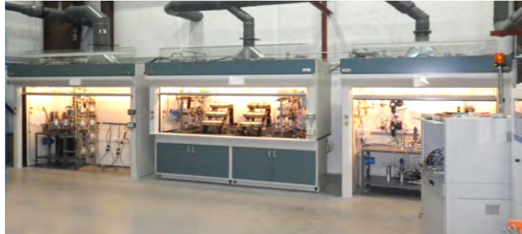
Top image: Test cells for exposing elastomer samples to simulated well conditions.
