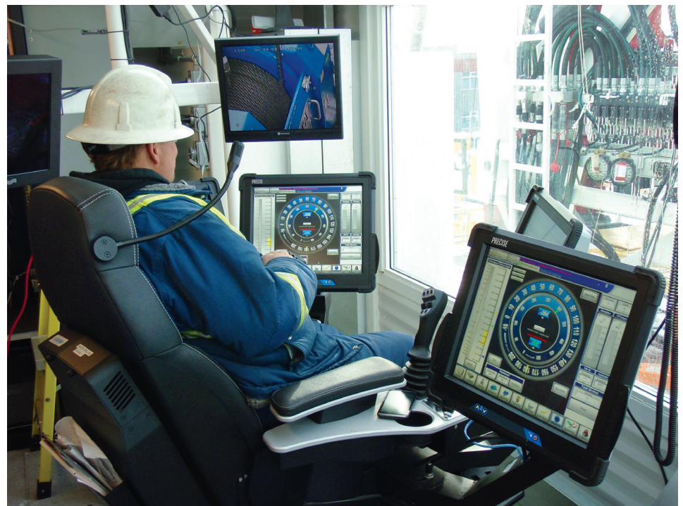
Every Schlumberger driller's cabin includes the PRECISE system, which enables the entire rig to be controlled from a single location.
