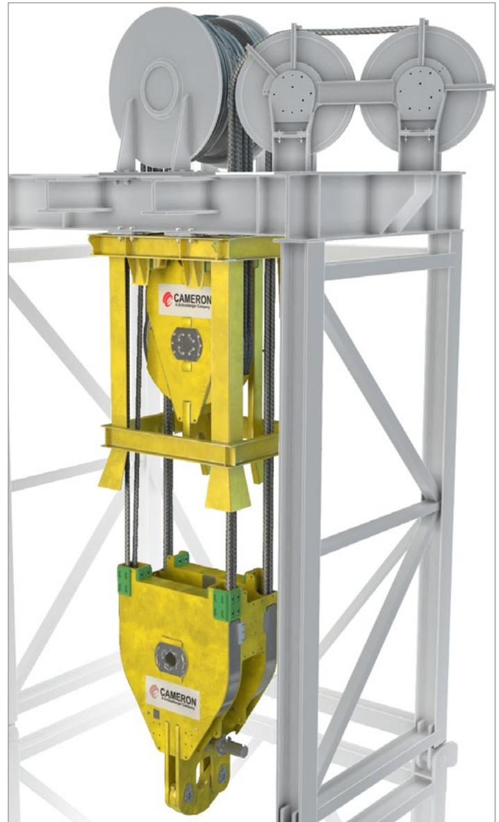
*The multispeed traveling block comprises two primary sections—the inner and outer cluster. The inner cluster is locked for fast mode and then reengaged to slide into the outer cluster for added lift capacity.*
