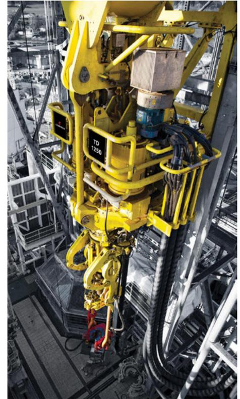
*The TD-1000-AC-2M top drive has a modular, customizable design that helps meet critical drilling objectives in a range of applications.*
