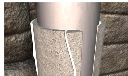
*The cement matrix remains active after the cement has set—for as long as there is cement in the annulus.*
