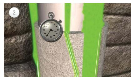
*The self-healing matrix reacts to create a complete hydraulic seal across the annulus.*
