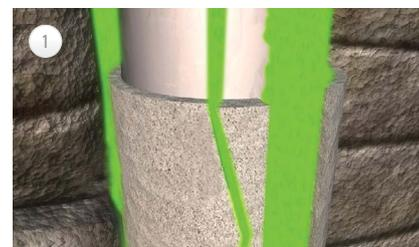
*Exposure to hydrocarbons initiates the self-healing response when and where it is needed.*
