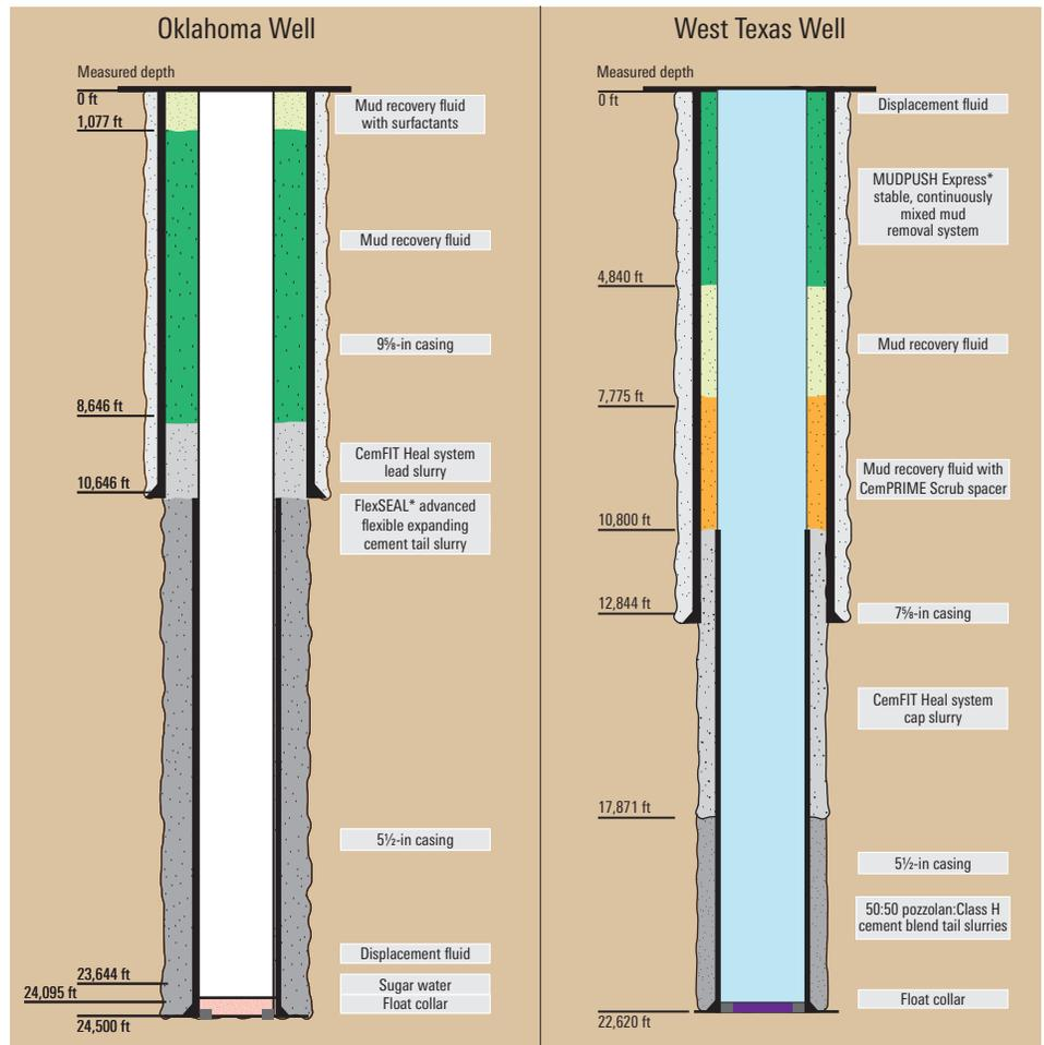
*In Oklahoma, using a relatively small volume of CemFIT Heal system as a lead slurry cap maintained well economics while eliminating SCP.*
