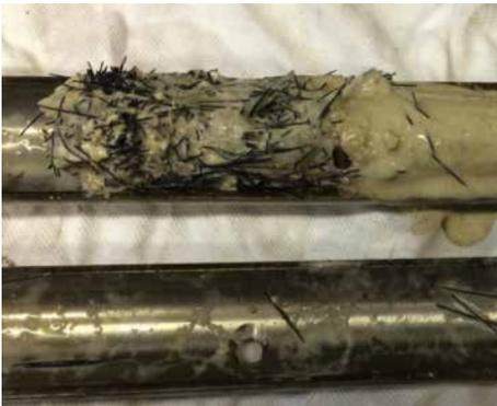
Losseal Natural Fracture treatment plug found in the wireline coring sample.
