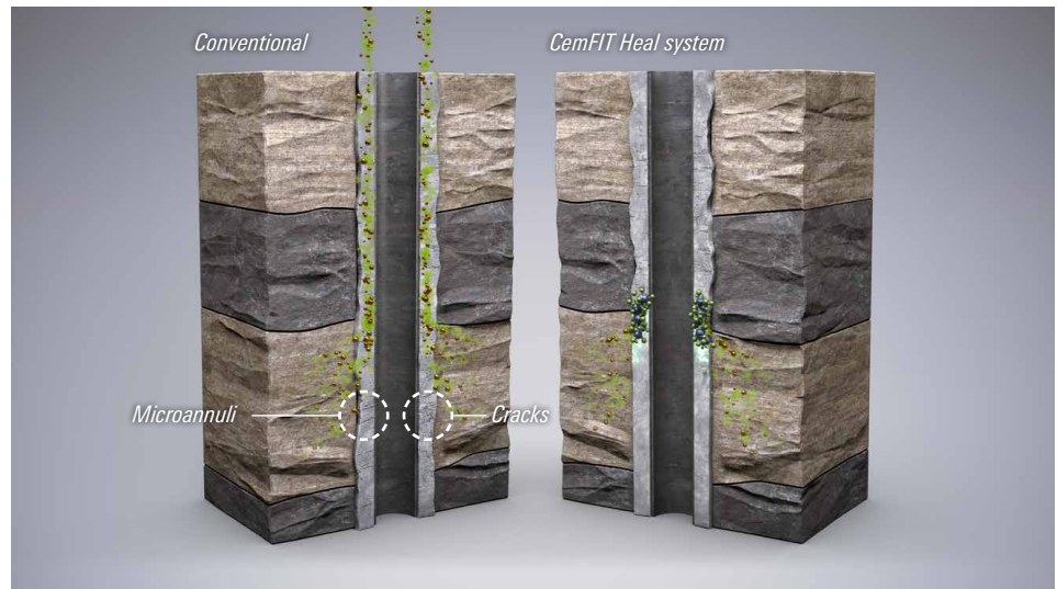
Conventional cement barriers (left) can develop cracks and microannuli caused by pressure changes and other stresses, allowing fluids to flow between zones and rise to the surface. The CemFIT Heal system (right) responds to any contact with oil or gas by automatically repairing and sealing itself.
