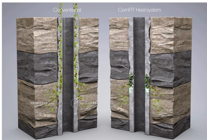
Conventional cement barriers (left) can develop cracks and microannuli caused by pressure changes and other stresses, allowing fluids to flow between zones and rise to the surface. The CemFIT Heal system (right) responds to any contact with oil or gas by automatically repairing and sealing itself.
