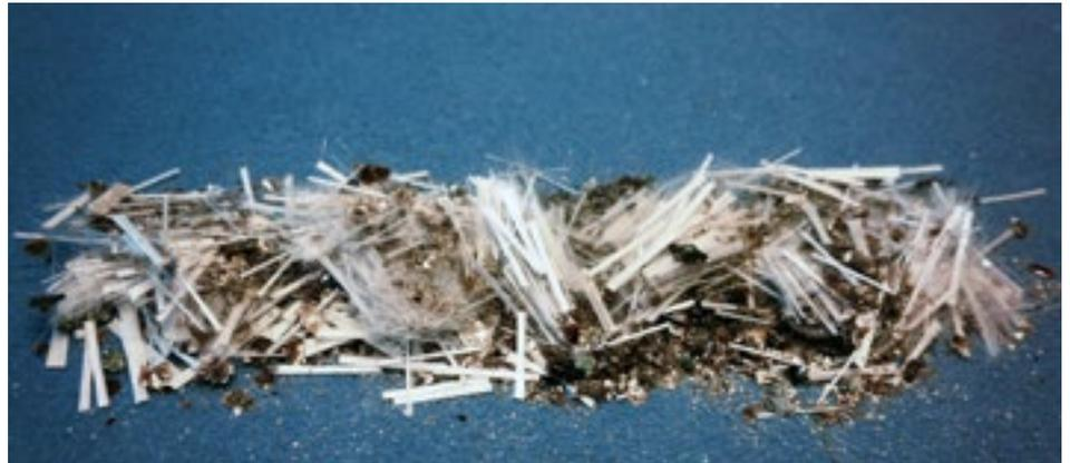
*The CemNET+\* engineered treatment for lost circulation features lab-tested fibrous material that can pass through 8/32-in (6.35-mm) bit nozzles to plug slots as small as 1/16 in (1.6 mm).*
