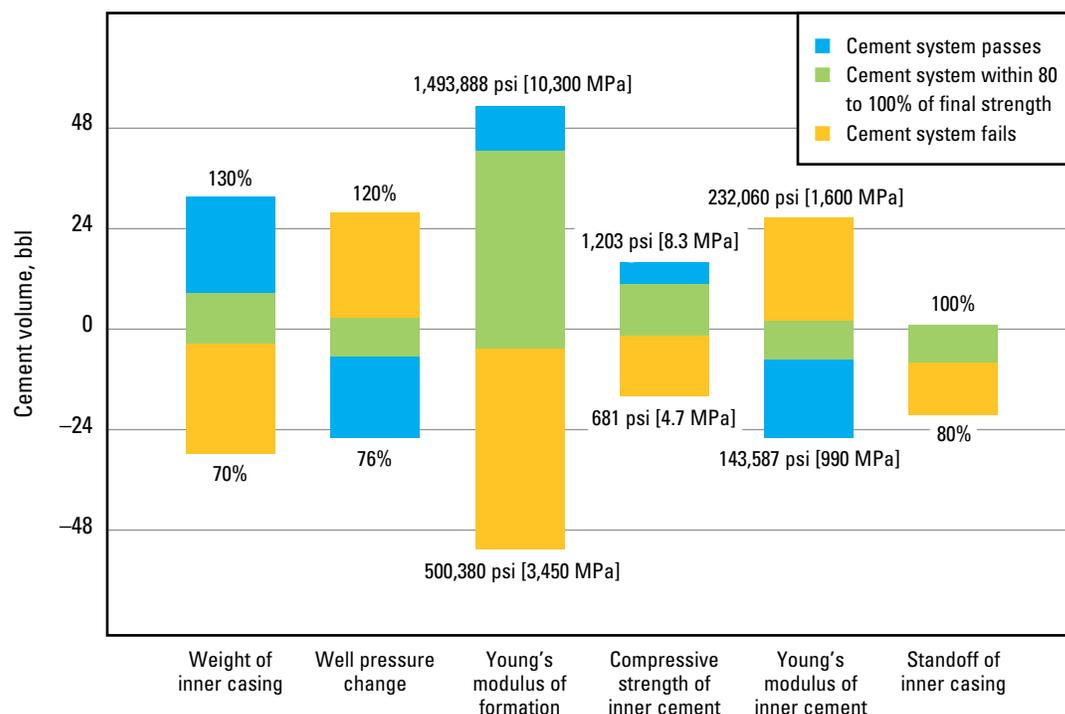
CemSTRESS sensitivity analysis, which allows like-to-like comparison of FlexSTONE systems with conventional and foamed cement systems (against the variance of numerous wellbore parameters).
