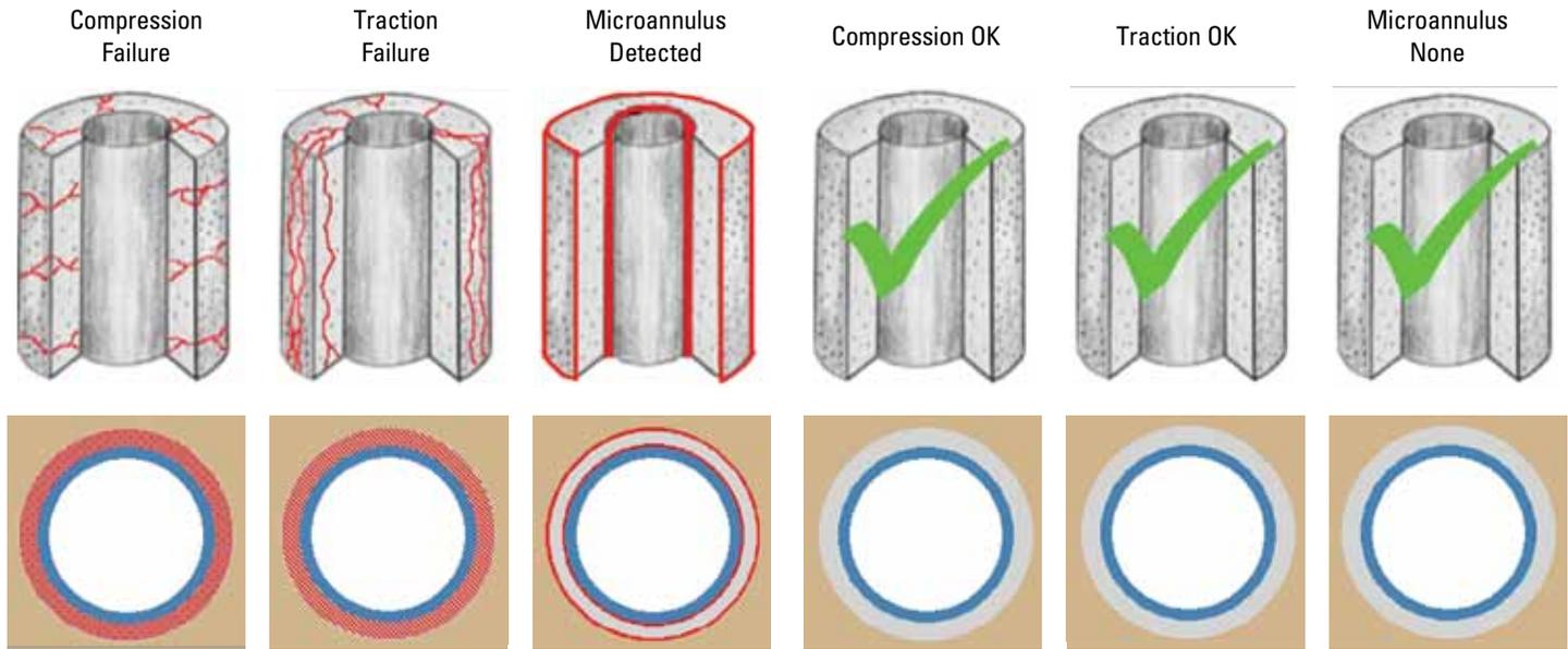
*Nonoptimized 16-lbm/galUS [1,917.2-kg/m<sup>3</sup>] cement system with Young's modulus of 1,160,301 psi [8,000 MPa]. The well cross sections (bottom) indicate various failure modes.*
