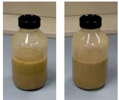
Left: 1.5-kg [12.5 lbm/galUS] slurry with 4% bentonite by weight of blend. Right: 1.5-kg slurry [12.5 lbm/galUS] with 2 kg/m³ ScavengerPlus stabilizer. Right sample shows a uniform appearance, with no settling. Pictures taken within 5 min of mixing.
