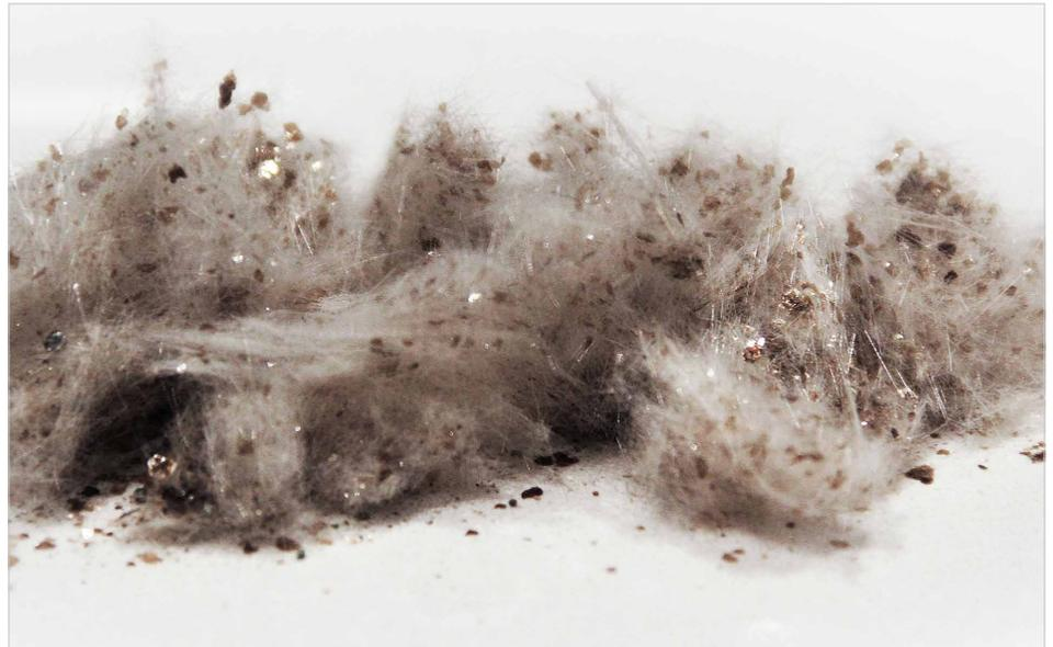
*The Losseal Microfracture treatment creates a compact, impermeable seal that plugs pores and fractures.*
