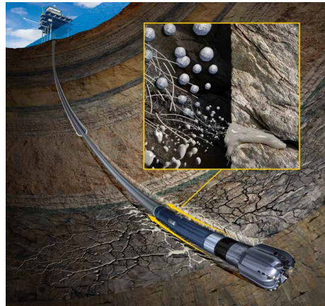
The Losseal Natural Fracture treatment creates an impermeable seal to cure losses.
