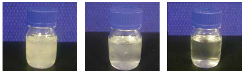
The Losseal Reservoir Fracture treatment's material in varying stages of degradation. The fiber system is stable for a configurable period of time then breaks down to allow for production, leaving the formation undamaged.
