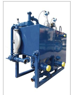
*The MUDPUSH Express stable, continuously mixed mud removal system uses a rapidly hydrating polymer that can be mixed on demand with a standard cementing unit, eliminating the requirement for additional resources.*
