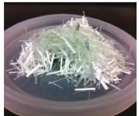
PressureNET lost circulation system combines the strength of vitrified shale (left) with a 3D network of CemNET engineered fibers (right)—effectively plugging lost circulation across a spectrum of fissure types.
