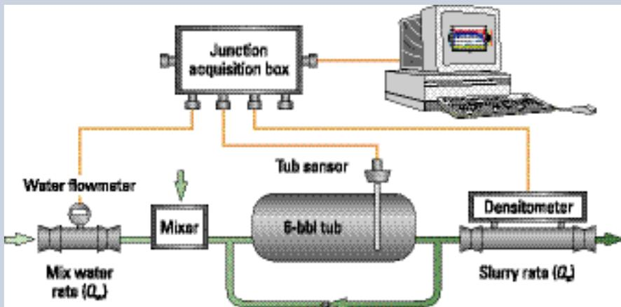
Windows-based software helps cementing crews monitor and adjust the blend whenever necessary using exactly the same procedures as in conventional slurry mixing. In a field application of the SFM system, 98 percent of the slurry volume has been maintained within 2 percent of the solid-fraction target.
