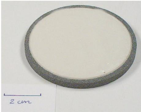
TemSEAL fluid forms a thin, compact filter cake to control fluid losses.
