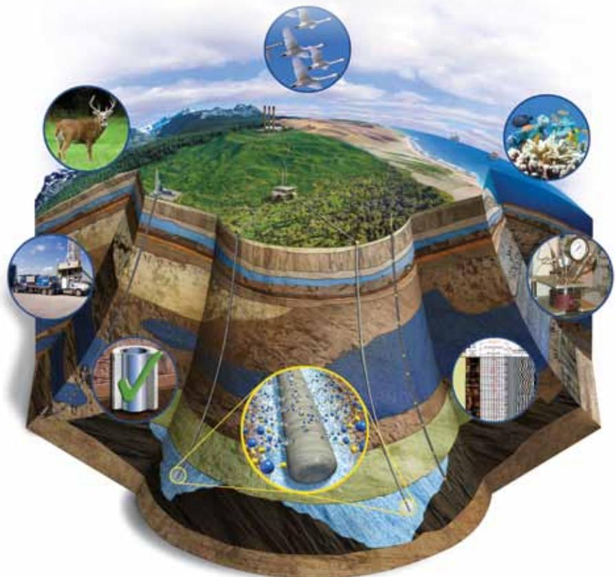
*ThermaSTONE cement is made of Portland cement, silica particles, and high-temperature-resistant particles. This cement is optimal for operations in the heavy oil market. Placement of the cement is on the casing string.*
