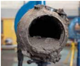
During the test, debris accumulated in and around the ball section.
