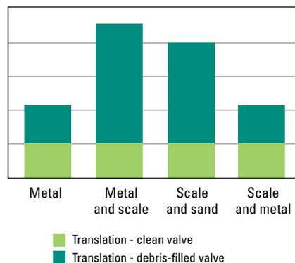
Left: Clean valves expended a constant amount of activation force, whereas the energy required by debris-filled valves varied greatly according to mixture type, in each case requiring from one to three orders of magnitude more than the clean valves.
