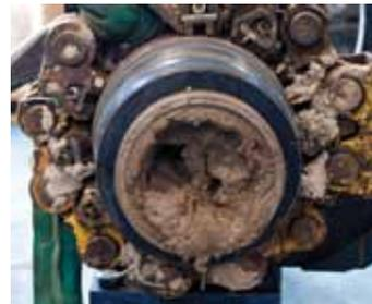
Debris completely clogged the mechanical section.
