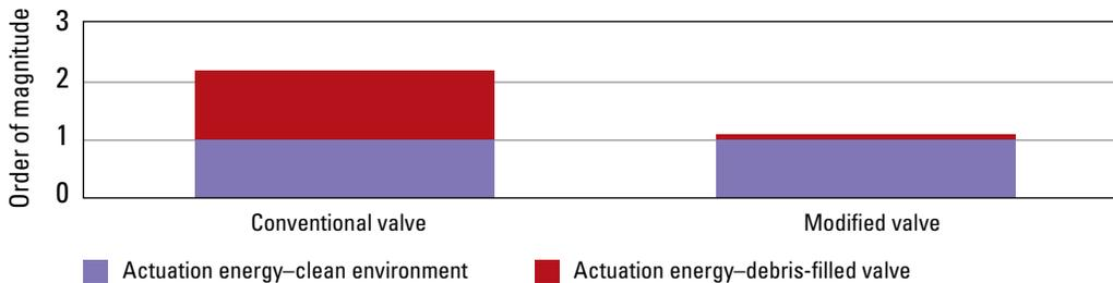
The force required to actuate clean and debris-filled conventional valves was compared with that required by clean and debris-filled modified valves. The effects of debris more than doubled the actuation force required by the conventional valve, whereas the effects of debris increased the force required by the modified valve only slightly.
