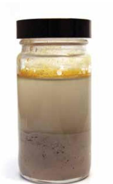
Over time, debris settles out of a fluid and becomes more dense, filling in voids.
