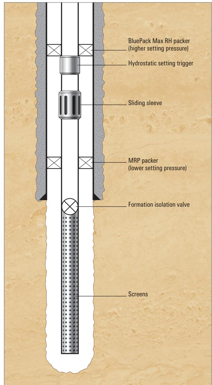
*Because of its customizable setting pressure, the BluePack Max RH packer was set after setting the MRP packer and circulating drilling mud out through the sliding sleeve, enabling a single-trip completion.*
