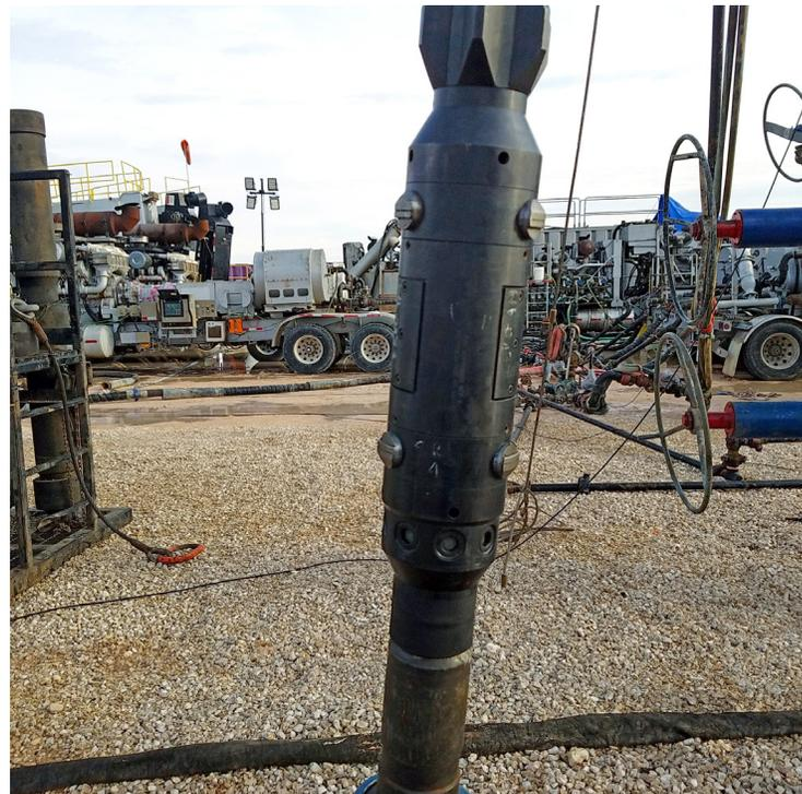
*CoilShift Precision CT frac sleeves reduced rig-up and rig-down times as well as the time between stages. In addition, they provided the flexibility for rigless zonal shutoff (e.g., for sand management) later in the life of the well.*
