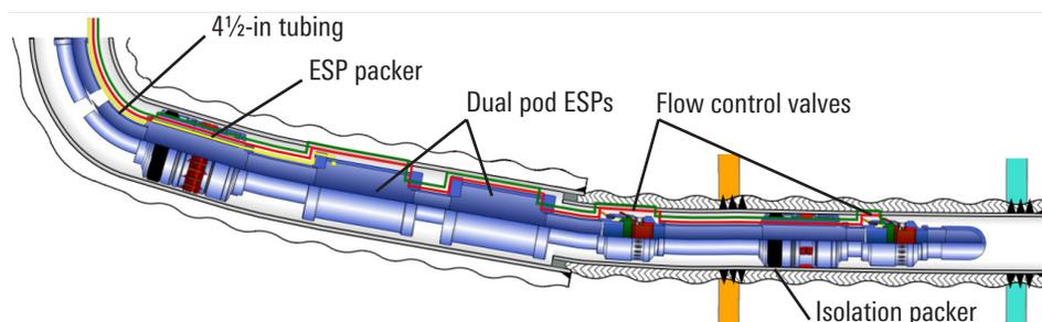
*The illustration shows the typical configuration for an intelligent completion deployed in an oil producer in the subject oil field. Together with the pressure and temperature gauges at the bottom of each ESP system, the flow control valves have significantly increased production and ultimate recovery. The pod system is a specially designed capsule that encases and supports an ESP system in a sealed environment.*
