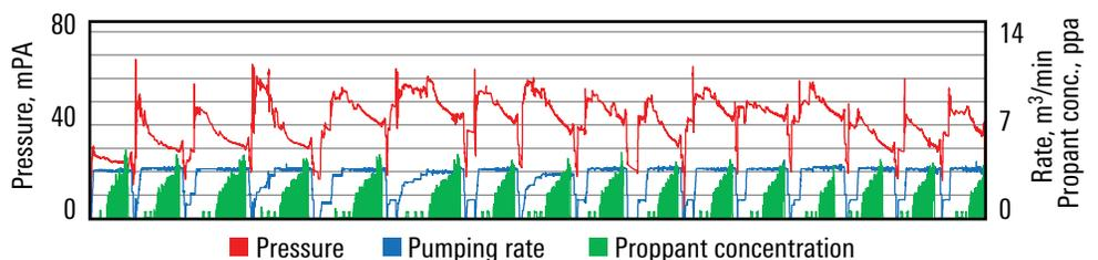
*The synchronized pressure response for the 16 stages shows that the pulses of locally sourced sand were injected effectively into the fractures, despite the high near-wellbore friction.*
