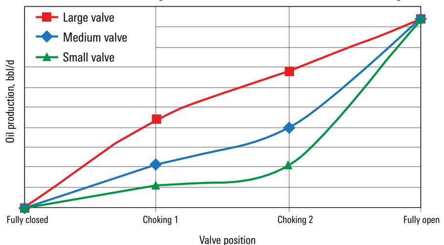
Nodal analysis was used to evaluate the optimal flow control valve sizing for three reservoir layers, with the objective of determining the zonal production rates as a function of specific tubing head pressure for three valve sizes and a range of choke settings. The figure shows the production rates in one zone based on three valve sizes and choke settings.
