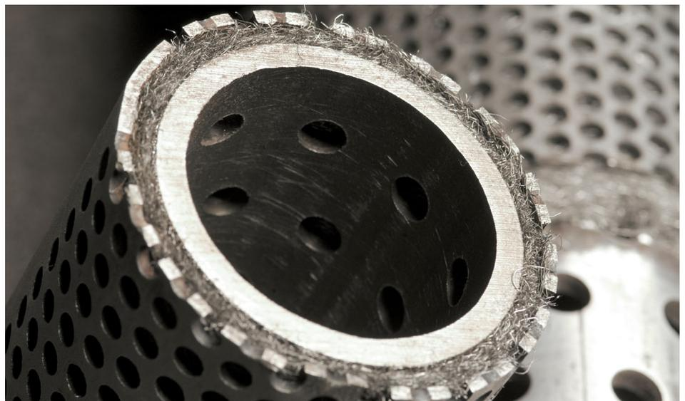
*MeshRite stainless steel wool screens created a partial exclusion filter, designed to retain the largest sand particles while allowing fine solids (<40 um) to pass through continuously, thereby retaining permeability and optimizing sand control.*
