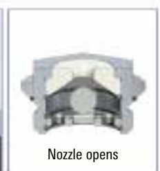
When the aluminum ball was dissolved using an acid-base treatment, hydrocarbons flowed from outside the annulus through the screen filter into the ICD housing and then into the basepipe through the nozzle.
