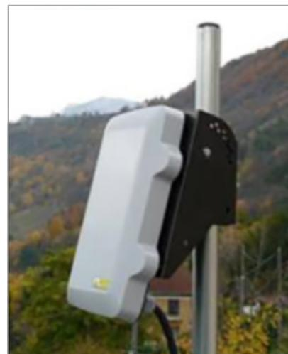
*A compact, self-powered WellWatcher Connect system collects data and transmits it to the operator's offices, reducing wellsite visits and improving reservoir management.*
