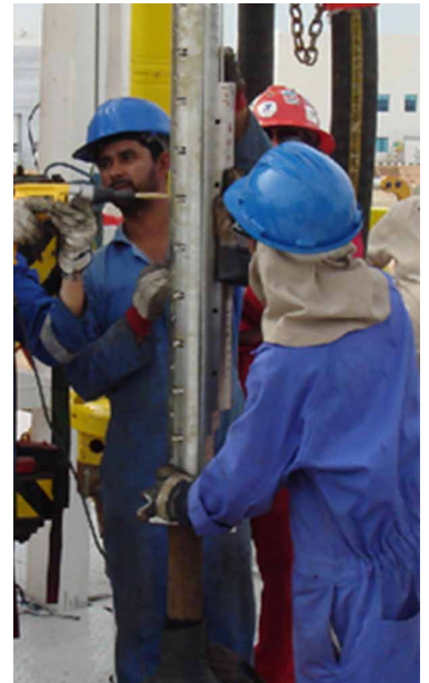
The WellWatcher PS3 passive seismic sensing system is deployed on tubing inside the casing.
