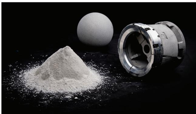
Fig. 1—The seat assembly and ball used in the new plug-and-perf system dissolve completely and predictably in temperatures of as low as 75°F (24°C), leaving no diameter restrictions to impede future operations.
